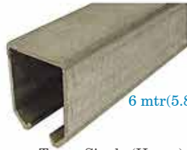
6 mtr(5.85 mtr.) Type : Single (Heavy) Size : for 350 kg. (57.5 x 67 x 2.0 mm)
